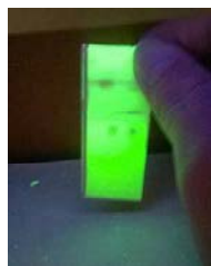
Fig. 12.1 Fluorescent TLC Plate Under an Ultraviolet (UV) Light
