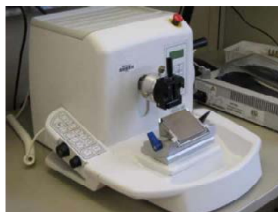
Fig. 9.2 Rotary Microtome Sectioning
