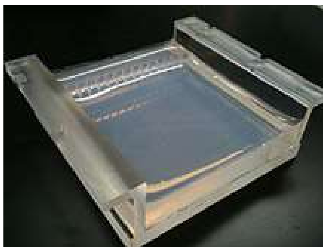
Fig. 11.5 An Agarose Gel Cast in Tray Used for Gel Electrophoresis
